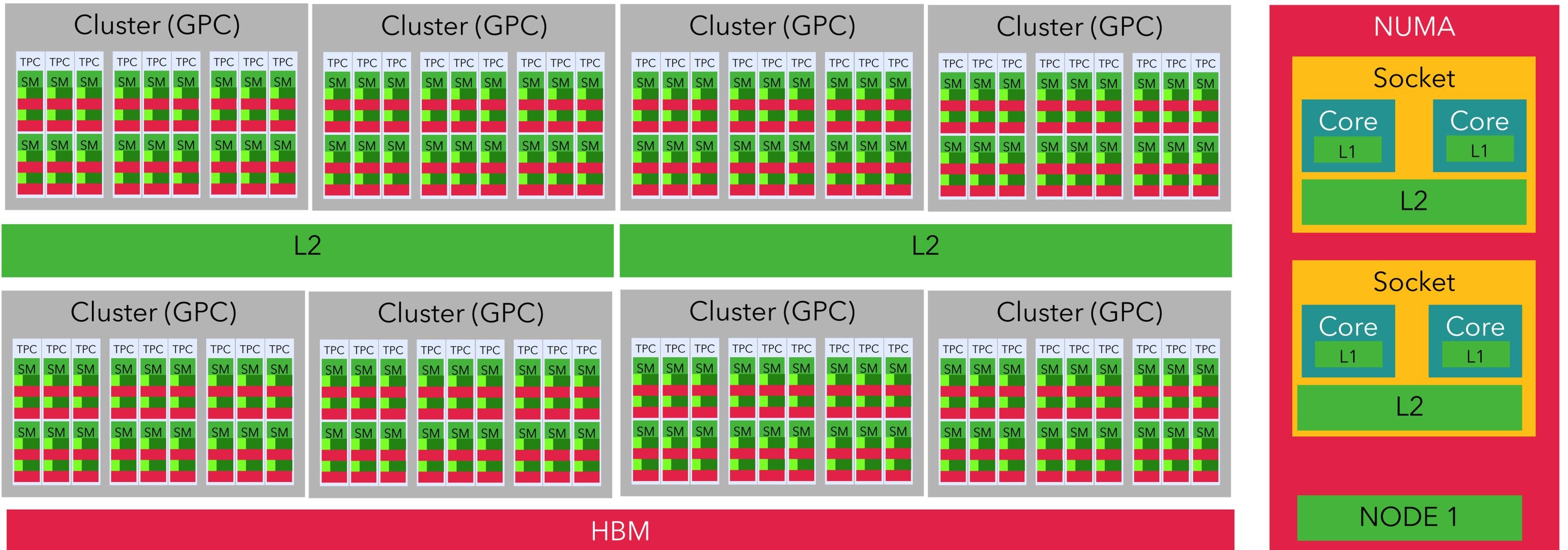
Current architectures also features a regular CPU over coherent memory
